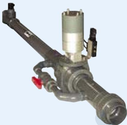
To safeguard the storage tank when using a compressed air feed from the feed tank, TECHAP offers its quick-acting fill protector as a complete unit (fast-closing valve including control unit, sensor and bypass valve with pipework) in nominal diameters DN 32, 40, 50, 65 and 80. There is a choice of the following materials: PVC, PP, VA (1.4571) and St.37.
